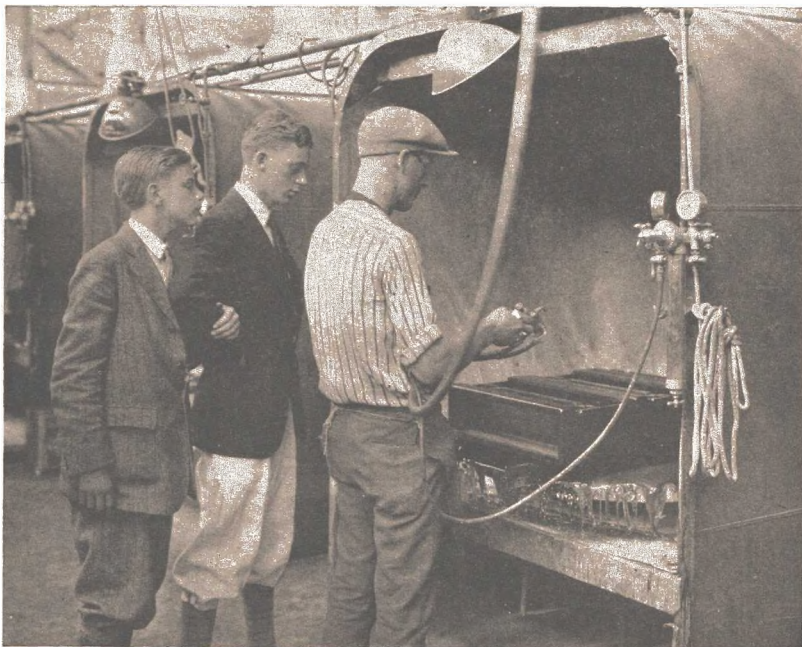
Spraying the Cabinets. Many men with brushes couldn't apply the lacquer as fast or as evenly as this one man does with his spray gun.
